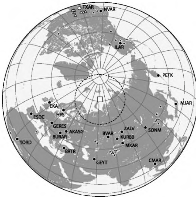
Figure 3. Locations of arrays (circles) and three-component stations (triangles) that recorded teleseismic P phases for the 11 October 2010 Novaya Zemlya event with a satisfactory SNR (see Fig. 2). The IMS seismic arrays are labeled. The stations at which the clearest depth phases are shown are displayed with white symbols.
